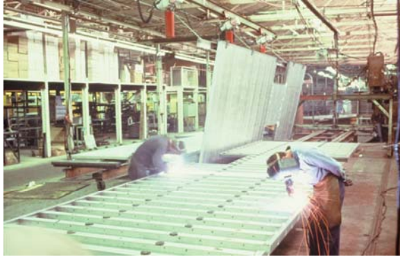
School Bus Sub-Floor
